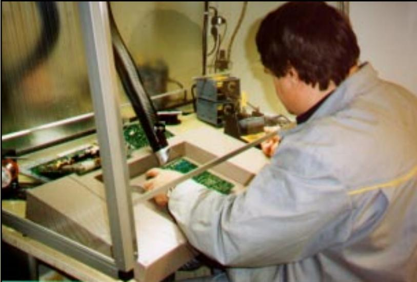
*This company repairs circuit boards. An extractor cabinet has been built for soldering and other jobs in which isocyanates are generated. It was designed by the staff together with a consultant in order to ensure its suitability for the various jobs involved. When the extractor cabinet is in use, no protective equipment is required. There are no measurable levels of isocyanates outside the cabinet.*
