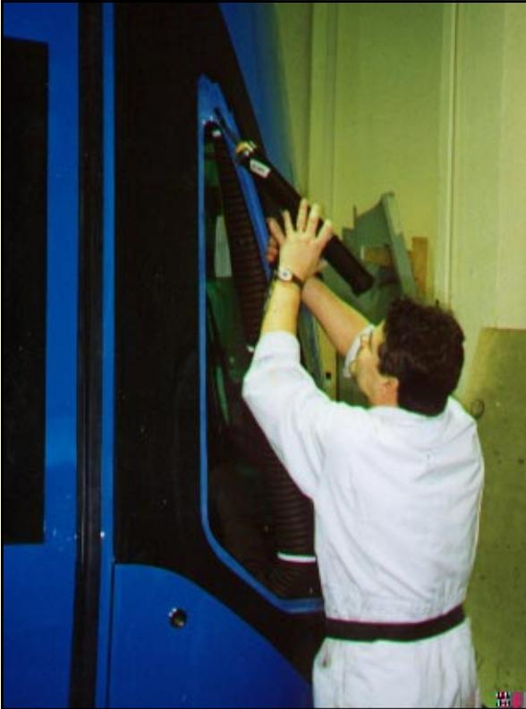
*PUR adhesive has been replaced by an MS adhesive (a Simson adhesive). The bonding process is the same as before, but no protective equipment is required and the process can be carried out even with other people working close by. This makes the bonding process more flexible – in the past, it was only possible to do it at nights and weekends.*
