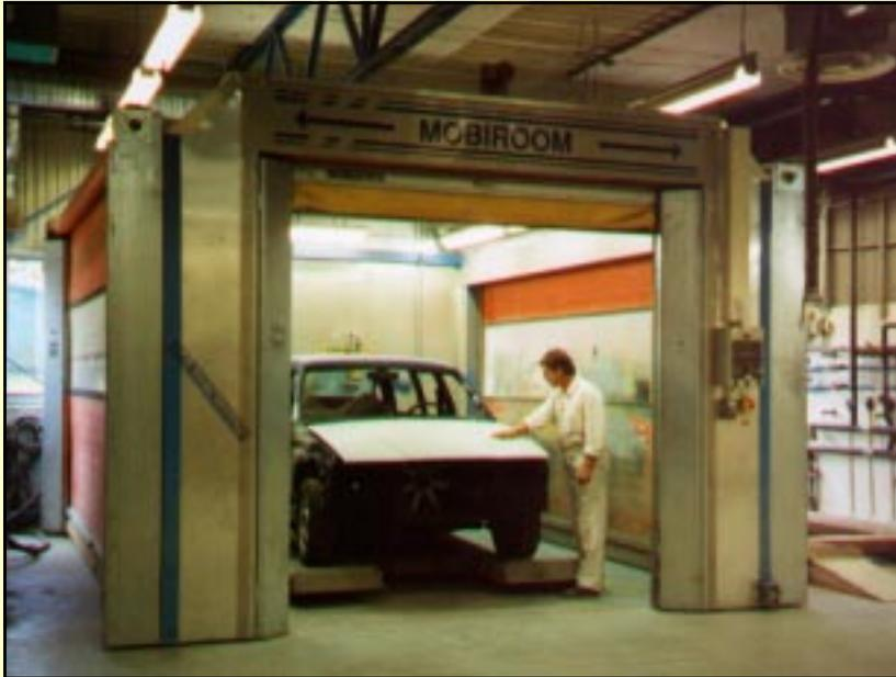
*A mobile booth for work involving isocyanates has been developed at this company. The booth can be moved around among ten workstations and is connected to a ventilation system that is fitted at each workstation. The mobile booth means that isocyanate work in progress does not disturb the people working alongside. Those working with isocyanates in the booth must wear a compressed-air face mask.*
